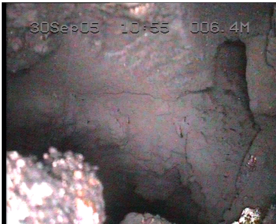
DRIFT 2 – Coal Mine working in BH3 as reviewed with CCT Camera
